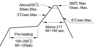
3.2 Reflow soldering should not be done more than two times.
