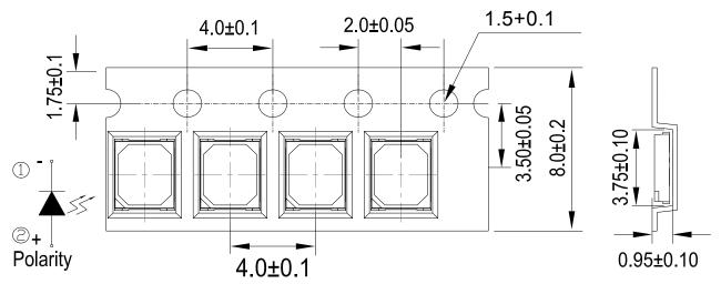
Note: Tolerance unless mentioned is ±0.1mm; Unit = mm
