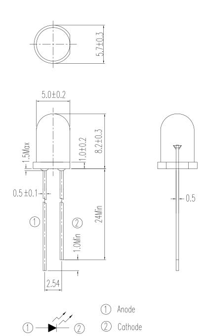
Note: Tolerances unless dimensions ±0.25mm
