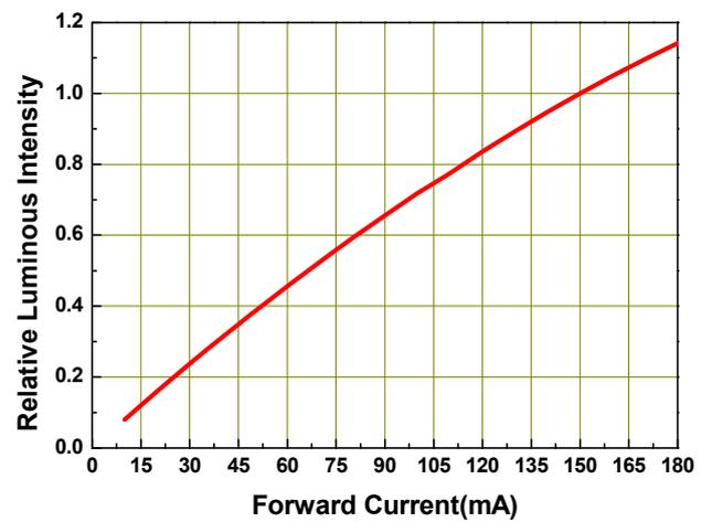
**Typical Electro-Optical Characteristics Curves**
