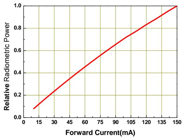
**Typical Electro-Optical Characteristics Curves**
