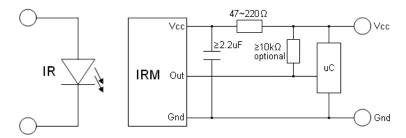
Fig.9: application circuit. The RC Filter must be connected as close as possible to Vcc and GND pins.
