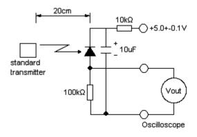
Fig.3 Measuring system
