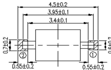
Note: The tolerances unless mentioned are  $\pm 0.1$ , unit=mm.
