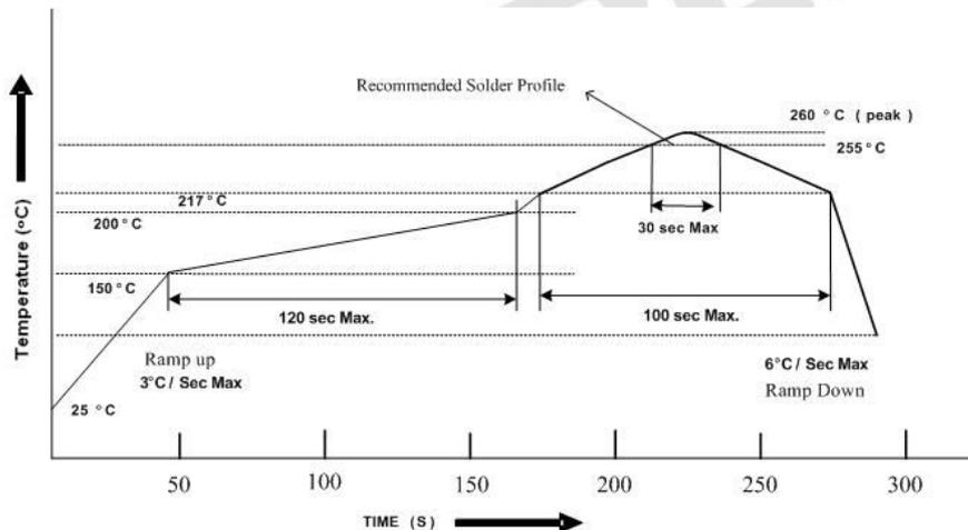
3.2 Reflow soldering should not be done more than two times.
