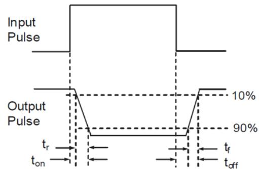
Figure 11. Switching Time Test Circuit & Waveforms
